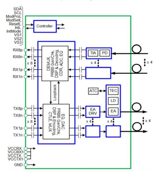
4x100G-LR1 QSFP-DD 10km Transceiver Module WST-QD4-PLR4-C
